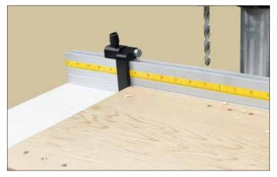
The convenient flip stop is designed to make repetitive and accurate drilling much easier. Simply insert the flip stop into the top track of the fence. Then line the flip stop up to the mark you need it to be placed and secure with the t-knob. Once the stop is positioned and secured, this will allow you to drill a hole at the exactly same location on different boards or you can move the stop to where ever you need it along the entire length of the fence.
