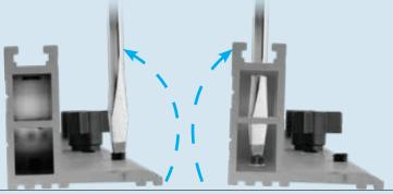
Once installed, the aluminum fence can be adjusted for squareness if needed simply by rotating two of the four set screws with a screwdriver as shown above. This eliminates the need for using those tough to find shims.
